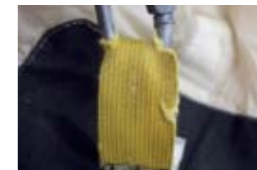
Attachment point frayed.
