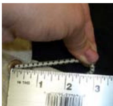
Shock cord loops 3 inches. Grommets in place.
