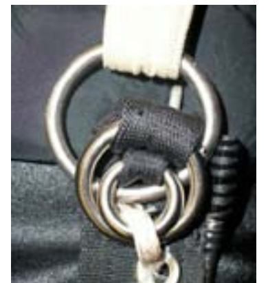
Large ring not round, around both smaller rings. Loop through both small rings.
