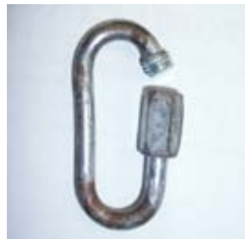
Link bent and rusted.
