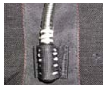
Tacking secure on drogue riser.
