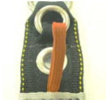
Securing loop in tact.
