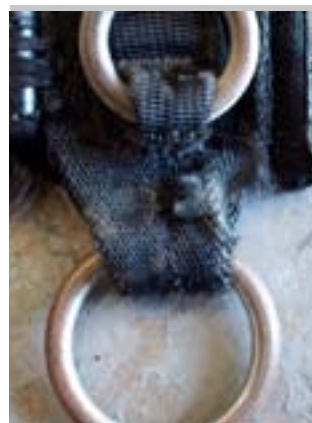
Webbing worn and fraying.
