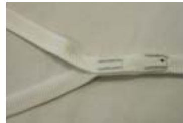
Bartacks secure, tubular in good condition.
