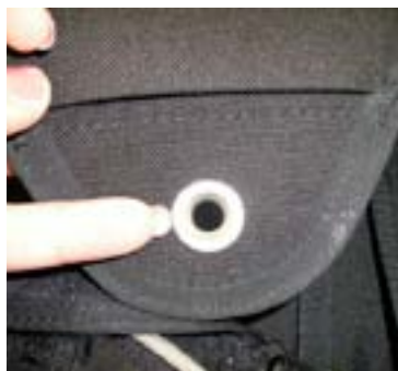
Fingernail doesn't slide under rim.
