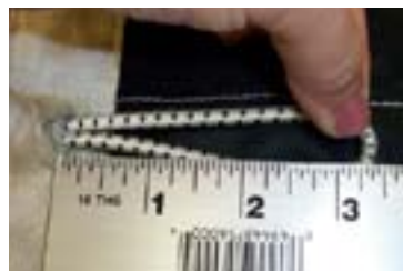
Shock cord loops stretched out. Missing Grommet.
