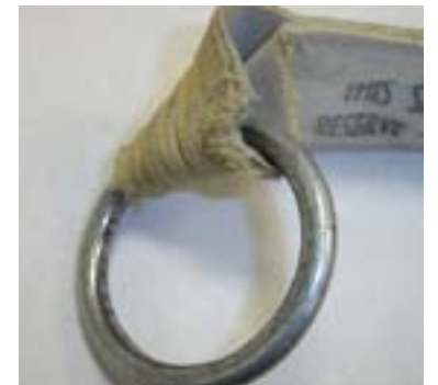
Fraying ring attachment point.
