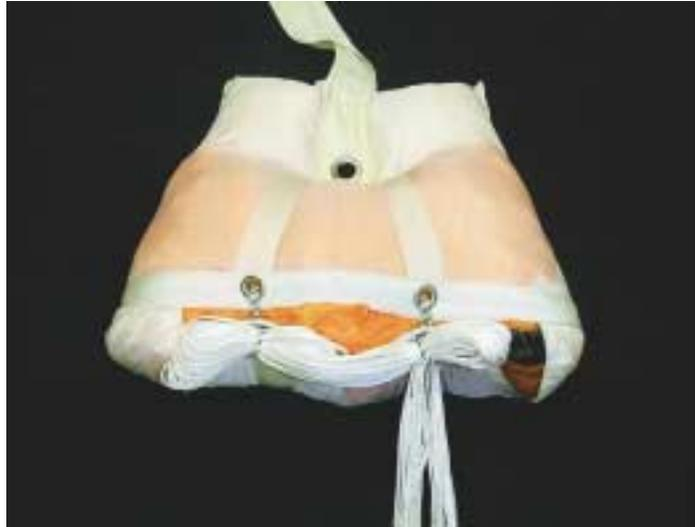
29. Rotate the bag onto its ears so that it is upside down and open the pouch on the bottom of the bag. Use the 1.5 X 6 inch pile Velcro®, mentioned in the *Required Tools* section, to cover the hook Velcro® on the bag side of the pouch so it will not snag the lines. S-fold the remainder of the suspension line into the pouch leaving about twelve inches from the bag to the links, then remove the pile Velcro® strips and mate the bag's Velcro® securely, being careful not to capture any lines.
