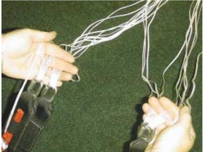
10. Walk toward the canopy pushing the slider ahead of you as you go. Continue until the slider is completely seated against its stops and cannot move any further. Ensure that the lines are tensioned evenly and that all are taut.
