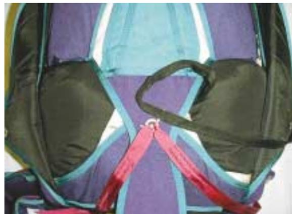
5. Stand the rig up vertically and close the riser covers by folding their plastic tongues into the riser cover pockets located on the inside of the yoke.
