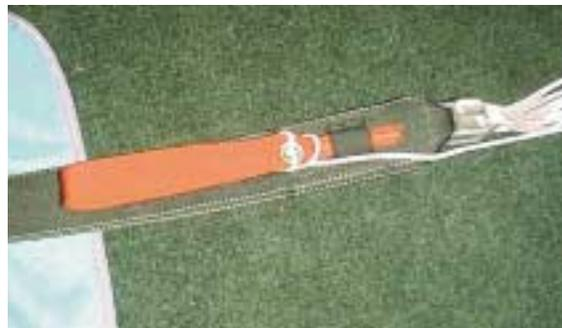
9. Standing near the rig, reach down and pick up the canopy's lines near the connector links. Use your fingers to separate the front riser lines, the rear riser lines, and the control lines.
