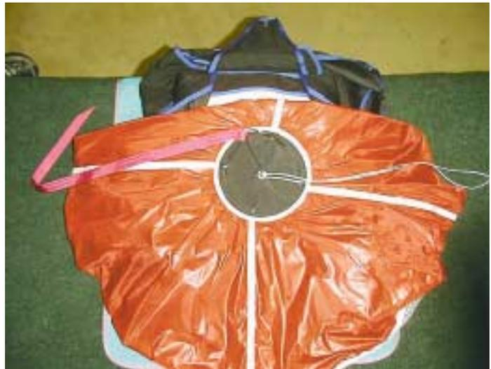
36. With the pilot chute centered, compress it fully and lock it with the temporary pin ensuring that no mesh or fabric is caught
