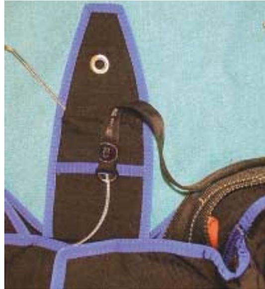
42. Close the top reserve flap and lock it closed with the temporary pin. Close the bottom reserve flap, remove the temporary pin and lock it closed with the ripcord pin.
