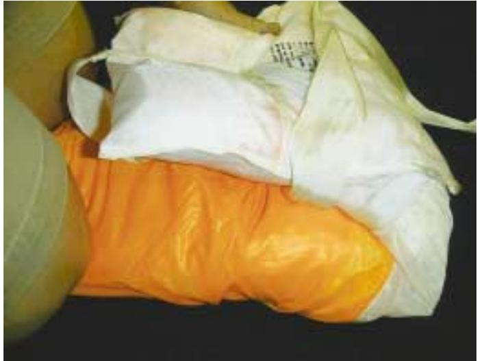
26. Now pull the bag towards you while folding it under the canopy to create an S-fold deep enough to fill the bottom of the bag below the ears.
