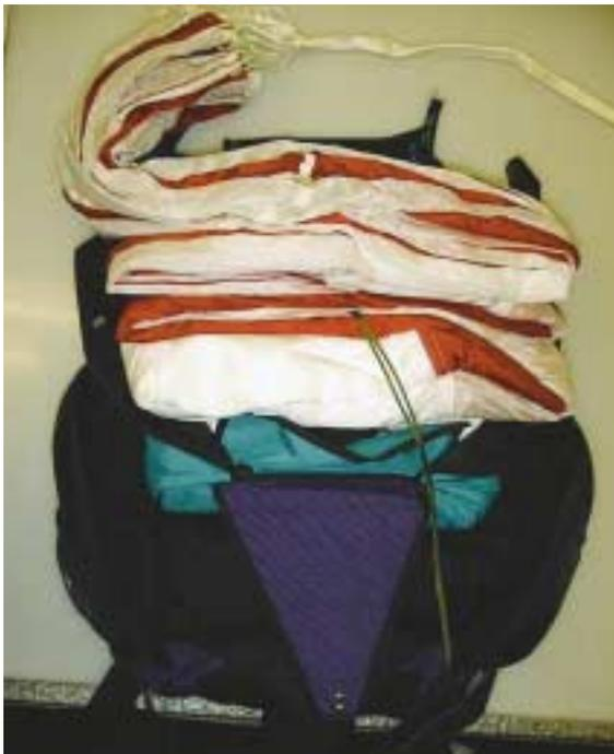
6. Position the apex of the canopy under the center of the top sub-flap with the bridle exiting to the right side.
