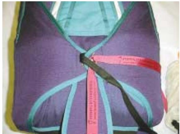
7. Tuck the bridle under the right side flap into the bridle flap of the container and then close the pin protector flap by folding it up over the side flaps and inserting it into the slot in the center flap.
