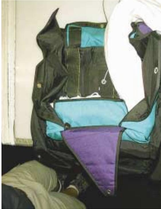
5. Continue S-folding the canopy toward the top of the container, keeping the folds slightly wider than the side flaps. The closing loop should extend between the fourth and fifth fold from the bottom.
