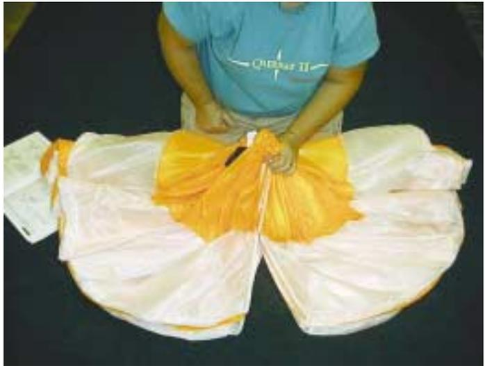
21. Fold the entire center cell straight under the base of the canopy and again kneel on it to maintain control. The canopy is now divided evenly into three sections, the center cell you are kneeling on, and the two ears which contain the outer three cells from each side of the canopy.
