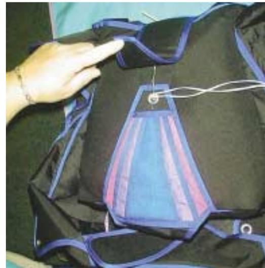
43. Seal the ripcord pin and record your work on the packing data card.
