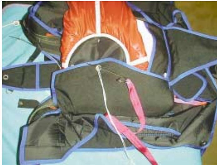
40. Now close the remaining right side flap and lock it closed with the temporary pin.
