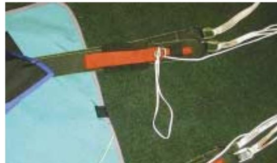
8. Set the right and the left deployment brakes by pulling the brake loop through the guide ring and then inserting the end of the toggle through the loop. Stow the excess control line under the toggle.
