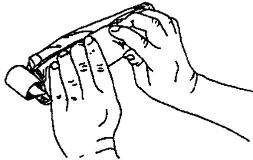
11. Slide the folded pilot chute and all excess bridle into the Spandex pouch located on the bottom of the container.
