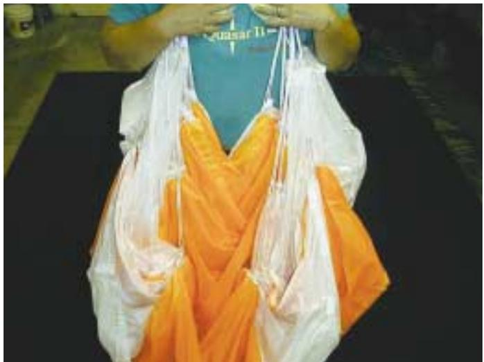
14. Ensure that the slider is still seated completely against its stops and push it down into the canopy between the right and left line groups. It should be folded in such a way so as to instantly catch air the moment its four corners are spread.
