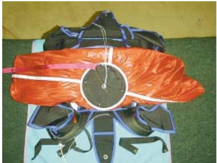
37. Spread the pilot chute's canopy so that it lies flat. Starting at the top, roll the fabric down to the base of the pilot chute and tuck it under the cap.
