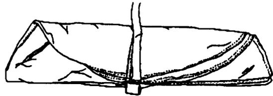
10. Fold the pilot chute in thirds and then roll it into a tight cylindrical shape.
