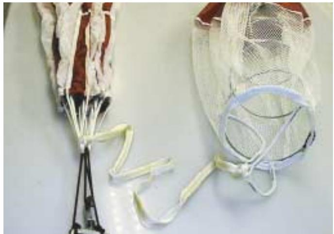
2. Attach the bridle to the canopy's apex with a lark's head knot as well.
