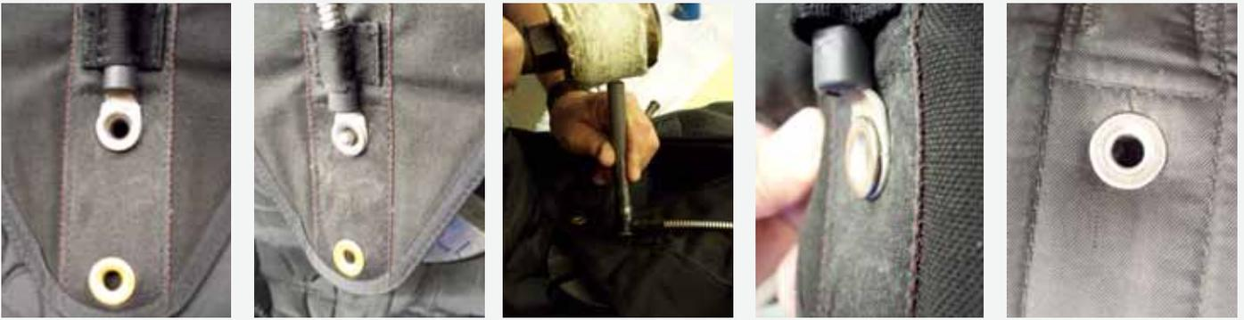
Place grommet through terminal end of housing and cover flap. Set in place. Depending on your grommet setting tool you may need to invert grommet and washer, should that happen the washer spurs need to be flattened prior to setting.
