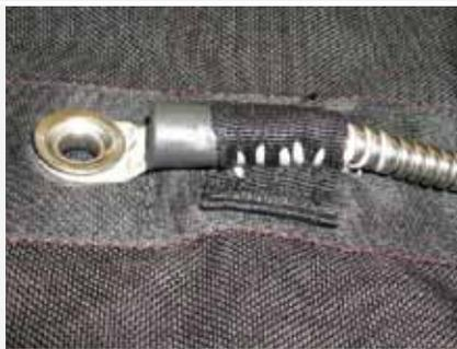
Make three more turns around housing and tie off to hold in place. Cut excess hand tack thread.
