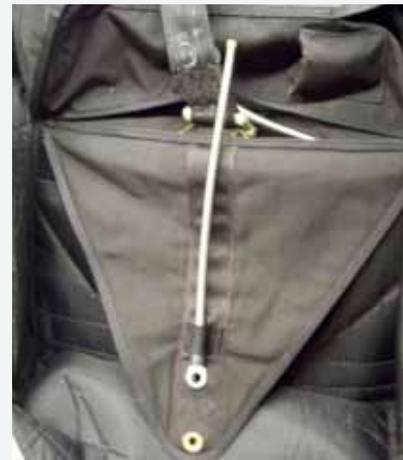
Place new housing with terminal end through drogue loop, positioning the terminal end of housing over original grommet hole.
