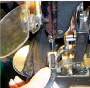
Using Type E thread Bartack, or make four passes with a medium duty machine, to attach loop to riser at 5/8' mark.
