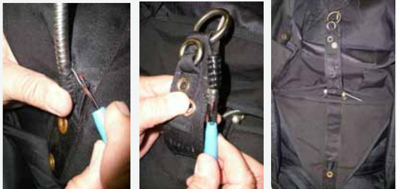
To begin modification the current housing needs to be removed. Make sure to avoid damage to drogue riser and drogue loop when removing hand tack.
