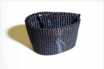
Taking a 2 3/4 inch piece of 1" Type IV create a 1' loop and mark at 5/8' from outside edge.
