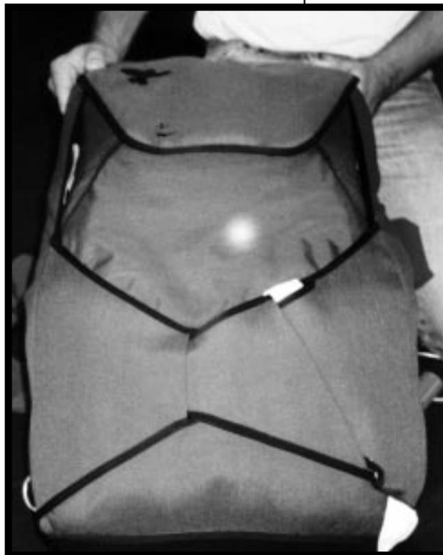
New internal and external flaps and closing pin keep the main deployment bag contained until the drogue is actually released. The drogue bridle is now covered with its own flap as well.
